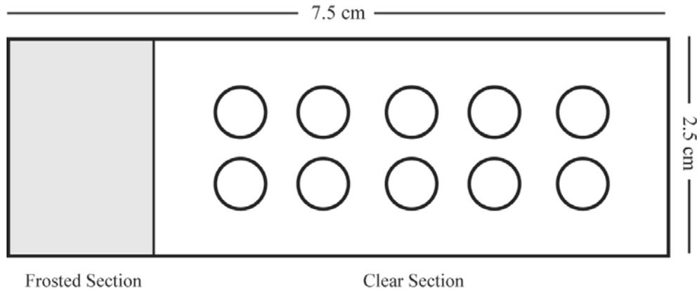
**Top-down view of a frosted microscope slide** - Each circular region encompasses the approximate area of a visual field. A total of twenty visual fields on both sides (front and back) of the slide piece are examined. Dimensions of an actual microscope slide may vary. Not all brands have identical slide dimensions. Figure is not drawn to scale.
